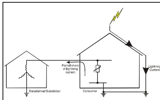
**Figure 1** 10/350 µs Coupling Mechanism as defined in IEC 61312-3 for a typical domestic facility
