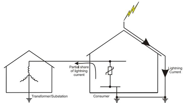
*Figure 1 Typical domestic facility as shown in IEC 61312-3*
